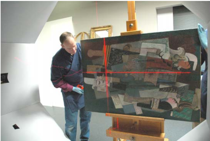
Figure 1: Oil paintings are not 2D images, but “very short sculptures” of many layers, and computational photography methods can reveal them. I developed this rig for low-cost 4-D lighting / capture (funded by NSF, NU) during my collaboration with the Art Institute of Chicago. We found pentimenti (‘regrets’ or hidden revisions) in several paintings, to augment X-ray, UV fluoroscopic, and IR studies. For example, in Pablo Picasso’s “Untitled (Man with Moustache, Buttoned Vest, and Pipe, Seated in an Armchair)” (1915) shown here, the rough paint textures include sand, dried paint scrapings, and possibly even coffee grounds. The black-and-white jester’s cap on the man’s head (left side) completed a series of revisions that included a curled-brim, bowler-style hat!
