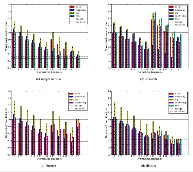
Figure 3. Normalized execution time for is, strsearch, bitcount, and dijkstra; showing the baseline performance and with three code optimizations: branch-rerouting, nop-padding, and loop unrolling plus brinc conversion. For nop-padding we examine two varieties: nop - which applies nop padding following any instruction capable of stressing critical path circuits versus selective nop, which inserts nops more judiciously.
