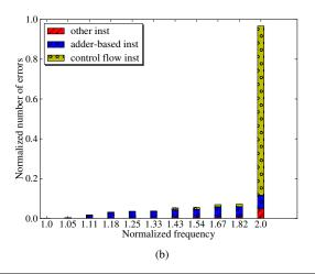
**Figure 5.** Failure counts categorized by type of failing instruction for the original strsearch benchmark and the strsearch benchmark with the jump rerouting optimization
