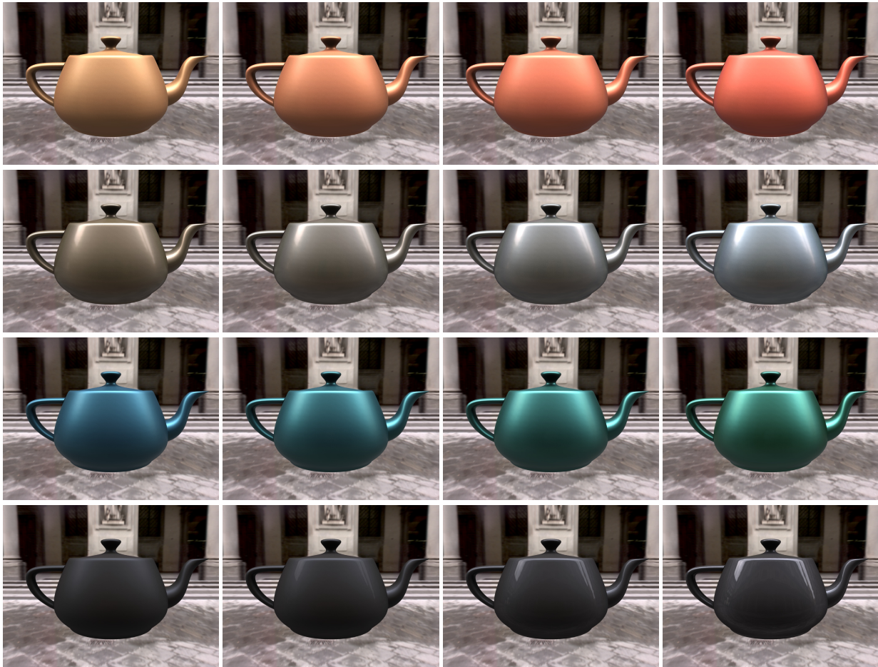
Figure 15: Navigation in the linear space. Each row corresponds to changing one parameter of the model. The first row shows an increase in the redness trait applied to the GoldPaint BRDF. The second row illustrates an increase in the silverness trait applied to the SpecularGold BRDF. Row three applies the gold-like trait to the BlueGlossyPaint BRDF. The fourth row shows an increase in the specularness trait applied to the BlackMattePlastic BRDF.
