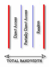
Overall scheme for division of bandwidth. The bandwidth may be broken into frequency channels to which appropriates schemes may be assigned.
