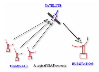
VSATs , very small aperture terminals , are small earth stations capable of receiving from , and sometimes transmitting to, satellites . They are an important part of the telecommunication world because they can provide a service directly to the user at virtually any geographic location covered by a suitable satellite beam.
