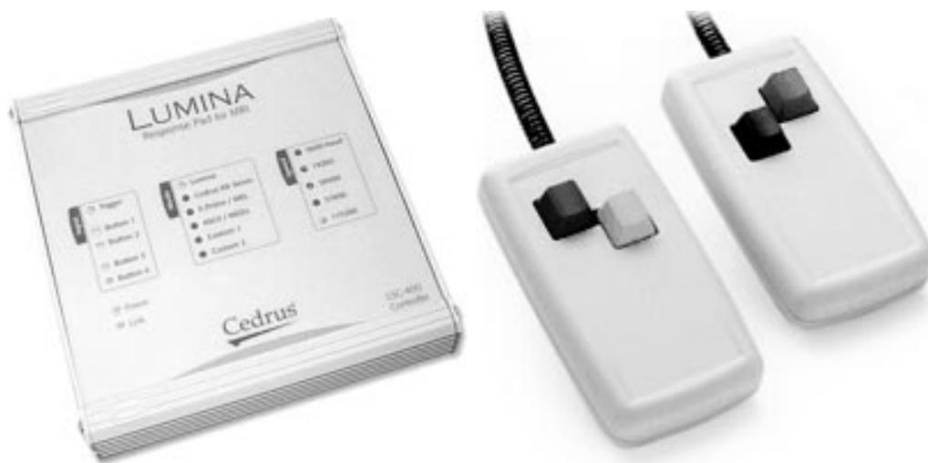
**Figure 3.6.** Left: The Lumina LP-400 controller. Right: The Lumina LP-400 response pads. This image is included here courtesy of Hisham Abboud and the Cedrus Corporation [1].
