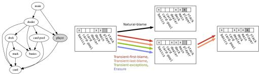
the dependency graph the paths taken by each mode through the configuration lattice
