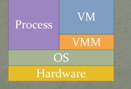
Type II VMMs that use *hardware* virtualization require modifications to the host OS (patches, or Kernel Driver as in KVM) to perform privileged virtualization instructions
