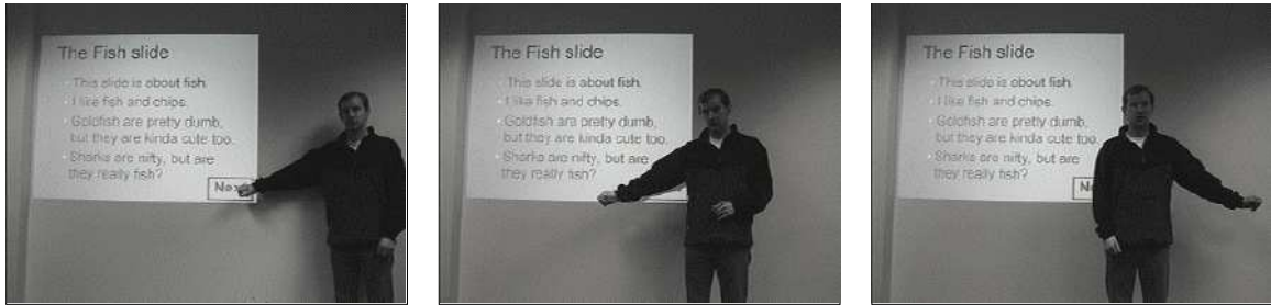
Figure 5.5: The three slide-control gestures: touch the next slide button, point right and point left.
