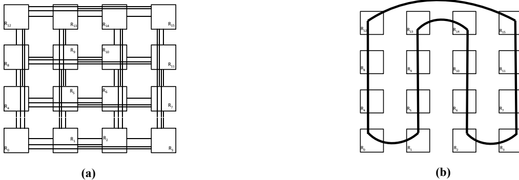
FIGURE 2: Electrical link (a) and serpentine waveguide (b) layouts for flattened butterfly topology.
