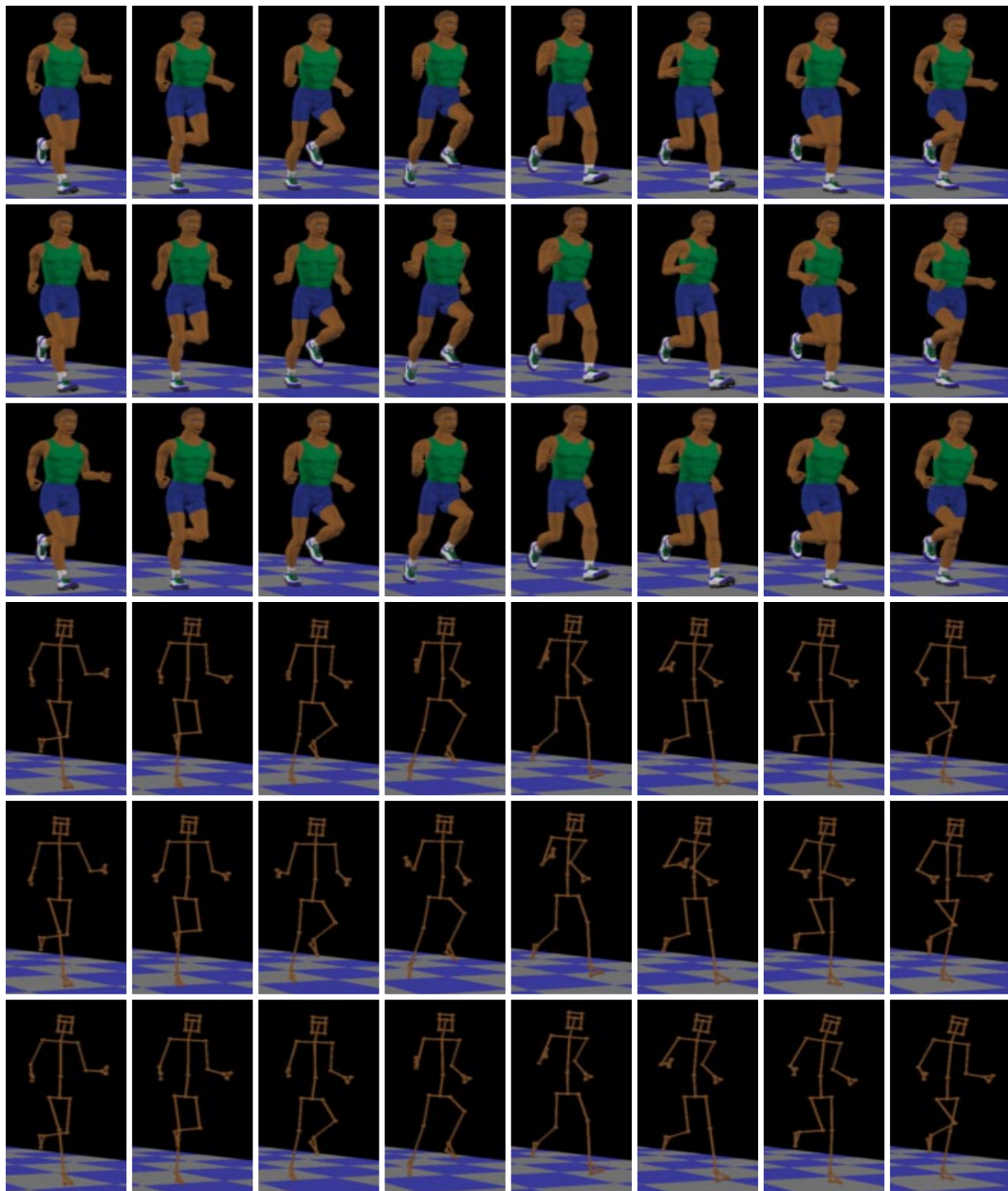
Figure 3: Sample image sequences from the animations used in the experiments. First Row: Original running motion rendered with the polygonal model. Second Row: Torso rotation with t = 1.0 . Third Row: Additive noise with t = 1.0 . Fourth Row: Original running motion rendered with the stick figure model. Fifth Row: Torso rotation with t = 1.0 . Sixth Row: Additive noise with t = 1.0 . Images are sampled at 0.067 second intervals.
