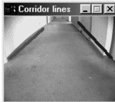
Figure 7.17: Line projections along the left and right walls of the corridor
