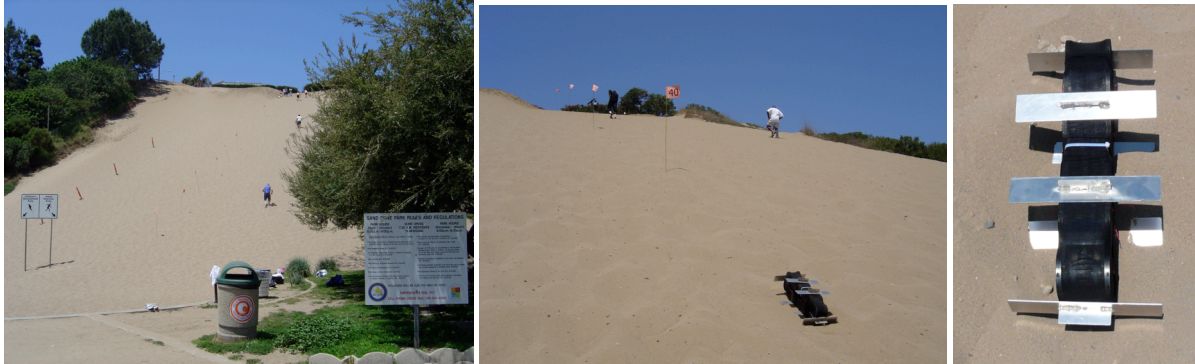
(a) The entire sand dune course. (b) SuperBot during climbing. (c) SuperBot with cleats and sand protection.
