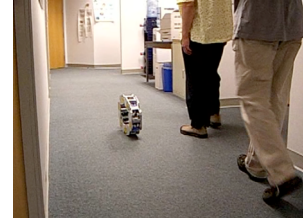
Fig. 3 A 6-Module SuperBot Rolling Track and the Changes of its Shape while traveling.
