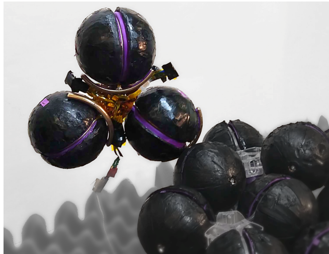
Fig. 1: FireAnt3D climbs atop a collection of its peers by flipping about strong connections it made using its 3D continuous docks. The robot attaches to like robots without alignment, allowing for simple locomotion.
