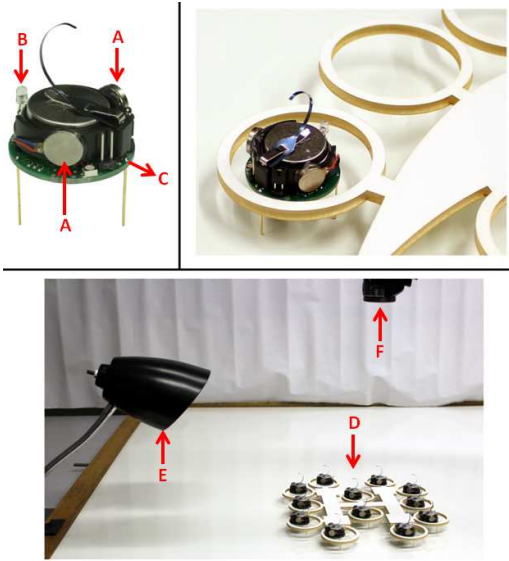
Figure 3: (Upper left) A single Kilobot robot, with motors (A), light sensor (B), and forward direction (C) marked. (Upper right) A Kilobot robot in an object gripping ring. (Bottom) Experimental setup showing a test object with robots (D), the goal light source (E), and camera tracking system (F).
