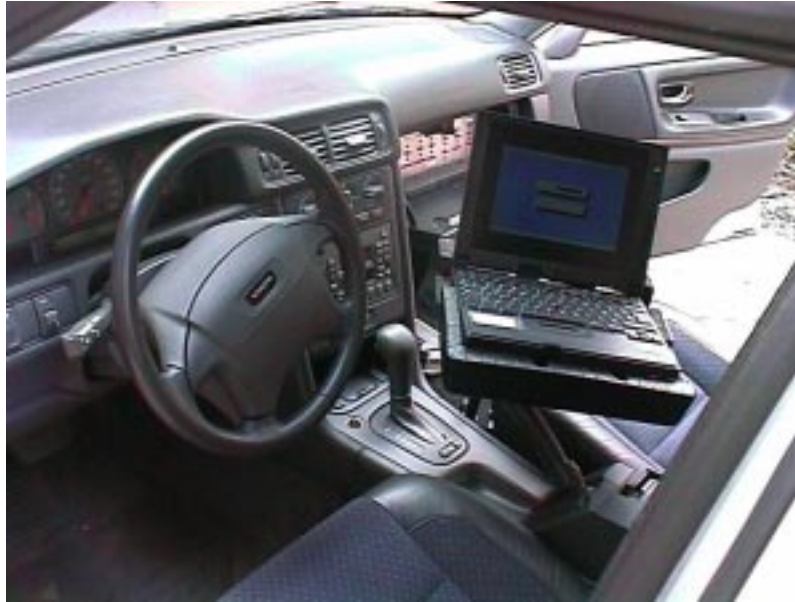
Figure 8.1: View of the Volvo Demonstrator Car showing the notebook connected to the ECU
