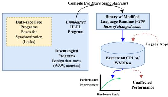
**Figure 1.** WARDen accelerates a broad set of applications without user annotation or static analysis while maintaining performance for legacy applications. Acceleration increases with hardware scale.
