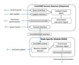
Figure 2: ConCORD's node-level architecture.
