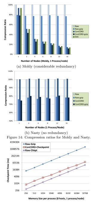
Figure 15: Checkpoint response time for a fixed number of SEs and nodes as the memory size per SE increases.
