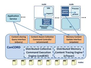
Figure 1: ConCORD's high-level architecture. Dashed boxes represent distributed components.
