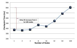
Figure 17: Checkpoint response time on *Big-cluster*. nodes, supporting the case that a scalable application service can be effectively built on top of the content-aware service command architecture.
