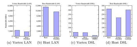
Fig. 8. Bandwidth measurements of clients hosted on DSL and LAN connections. (a) and (c) contain the performance results of a Vortex CSW, while (b) and (d) contain the performance results of the client machine. Measurements were taken under various traffic conditions and bandwidth is measured in kilobytes/second. Each figure shows the mean taken from 10 separate trials.
