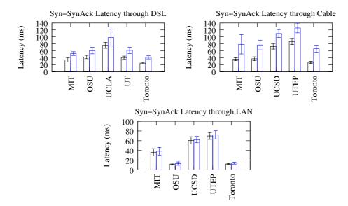
Fig. 9. Differences in latency between a local service and a CSW. Measurements were made by timing the Syn/SynACK sequence caused by the establishment of a TCP connection. Measurements were taken from various PlanetLab sites distributed across North America. For each site the latency of a local service is shown on the left side while the CSW latency is on the right.
