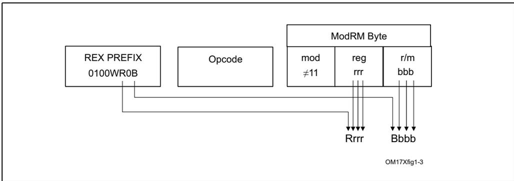
**Figure 2-4. Memory Addressing Without an SIB Byte; REX.X Not Used**
