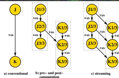
Allows pipelining and pre/post-computation
