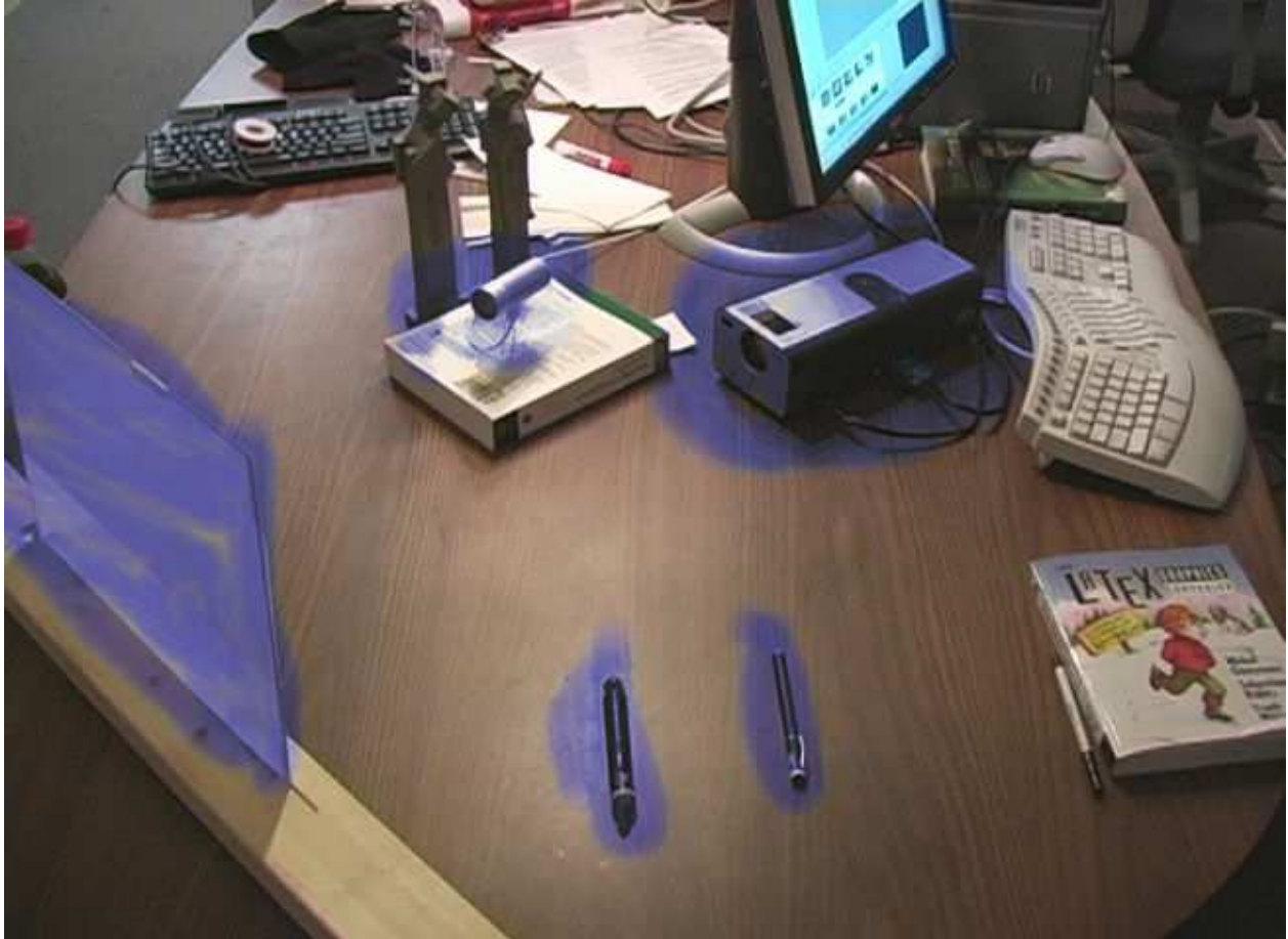
Figure 2.1: The back projection system, which consists of a plexiglass plate, projector, and webcam. Also highlighted are the drawing devices, the light pen and laser pointer.
