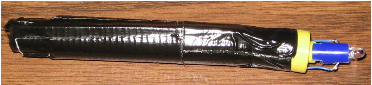
Figure 2.3: A pressure sensitive light pen, constructed out of an LED and two AA batteries.
