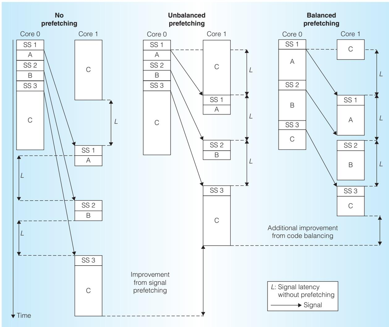
Figure 3. Importance of balanced prefetching. Without helper threads or balanced code scheduling, a parallelized loop with three sequential segments, running on a dual-core processor, might behave as shown on the left. With helper threads but no code balancing, signal prefetching reduces delay, as shown in the middle. Adding balanced code scheduling further reduces delay, as shown on the right.
