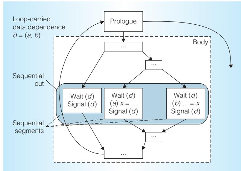
Figure 2. Insertion of  $Wait(d)$  and  $Signal(d)$  due to a RAW data dependence  $d = (a, b)$ . Sequential segments that contain only  $Wait$  and  $Signal$  operations handle dependences that span multiple iterations.
