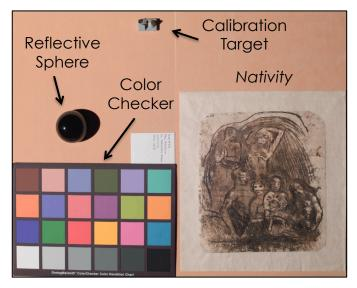
Fig. 7: The setup for capturing photometric stereo of Gauguin's *Nativity*. A color checker for color calibration, a 3D calibration target for 3D surface calibration, a reflective sphere for calibrating light direction, and the work of art.
