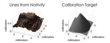
Fig. 12: Comparing the 3D reconstruction with the 3D calibration target. The height of the cone in the calibration target is approximately 10mm. The surface reconstruction of *Nativity's* protruding lines are approximately  $100 \times$  smaller, indicating they are on the order of  $100 \mu m$  in height.
