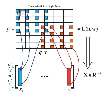
Figure 4. Block sampling of a canonical plenoptic image and lexicographically reordering into a vector. Here we show sampling from a block with  $B_u \times B_v = 4 \times 4$  spatial samples, and  $B_p \times B_q = 3 \times 3$  angular samples. With color included, the entire signal contains  $3 \times 3 \times 4 \times 4 \times 3$  samples and can be represented as a  $x \in \Re^{432}$  vector.
