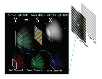
Figure 2. The Bayer filter used in a plenoptic camera causes gaps between the rays measured in each color channel. The area behind a single lenslet is zoomed in to show the effect of the Bayer filter on the captured light field. The bayer filter effectively applies a subsampling matrix S to the full-color light field X, producing the sensed light field Y. The sensed light field contains gaps: some of the rays in each of the color channel are not measured.
